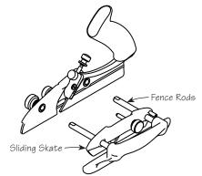
Figure 3: Installing the sliding skate.
