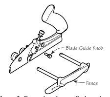
Figure 2: Preparing the small plow plane.
