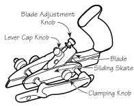
Figure 4: Blade installation.
